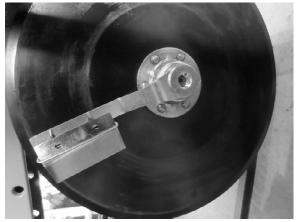
12. Replace and tighten the gauge wheel and arm back onto the row unit.
