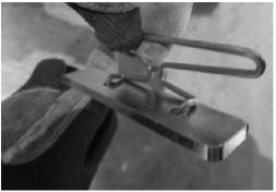
3. While the two tensioning wire posts are still vertical attach the blade lock by running the tensioning wire posts through the two holes in the blade lock.
