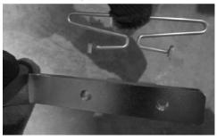
2. Insert the tensioning wire into the scraper arm by holding the tensioning wire vertical in relation to the scraper arm and pushing the two (2) tensioning wire posts through the two (2) receiving holes in the scraper arm.
