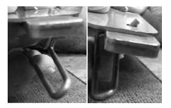
4. Push on the stainless tensioning wire so that the ends of the posts lie flat against the front side of the scraper arm and blade lock holding them securely in place.
